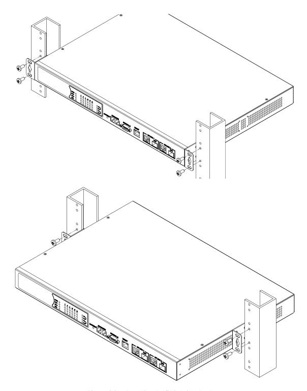
Figure 4-2. Installing the Switch in a Rack
